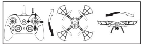
After you have the basics of flying, you're ready to learn flip and roll your drone. To perform a flip or roll, press the *Flip* button, make sure the drone is at least 3 meters o the ground and guickly push the Rudder, in either direction to make the drone flip or roll. Once the manoeuvre is completed, steady the drone.
