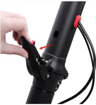
2. Fully open the release lever.
