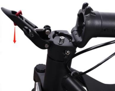
3. Open the scooter by accompanying the handlebar tube downwards.
