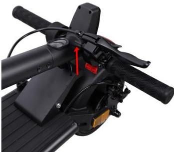
3) Close the lock lever located on the lower part of the handlebar support tube.
