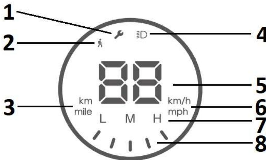
1. Service mode / error condition. Scooter failure. Please contact support.
