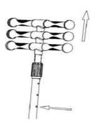
2. Press the metal lock on the handle, and then hold it while you pull up, or push down until the handle reaches the preferred height.
