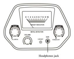
Note: The internal speaker is disconnected when you connect headphones.
