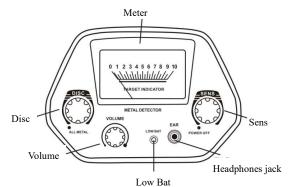
a. DISC – Rotate the control knob clockwise away from ALL METAL to get to DISC mode. The DISC mode comes with automatic ground balance. Rotate the control knob slowly clockwise to eliminate different trash objects. Rotate the control knob counter-clockwise towards the end to get to ALL METAL mode. The ALL METAL mode also comes with automatic ground balance. This mode used to find not only ferrous metals, but also non-ferrous metals (see more details below).
