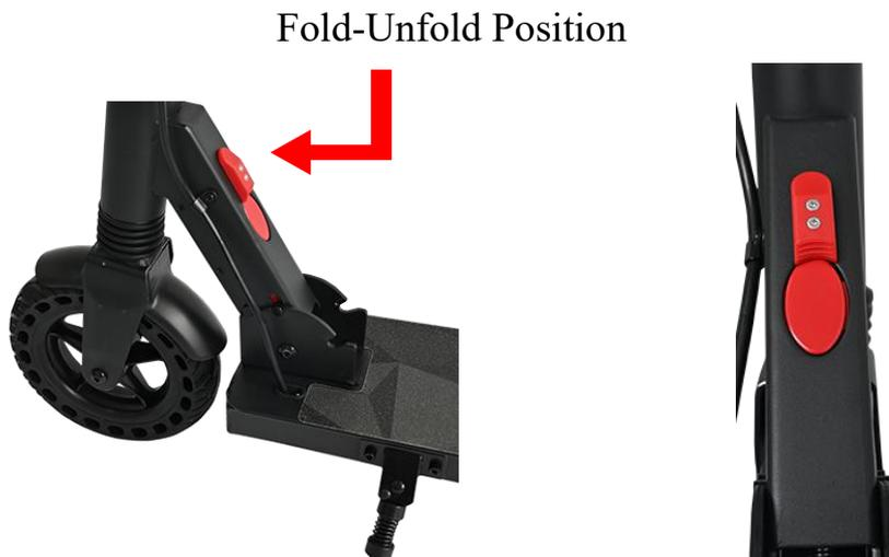
Push up and press the red button to fold or unfold the Electric scooter.
