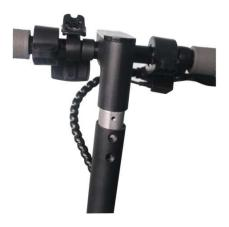
2). After matching the holes in the handlebar with those of the frame, insert the screws and tighten them well; repeat the operation also in the side opposite of the handlebar inserting a total of 4 screws.
