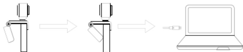
1. Turn on the Camera Mount and point the camera toward the front of the display.
