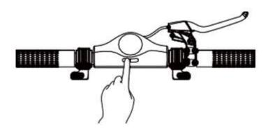
5. For safety, the rear drum brake must be used when driving at high speed. Use the right hand brake on the steer.
