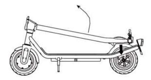
3) Raise the front pole and the pull up the folding wrench towards the upright pole and force it to lock.
