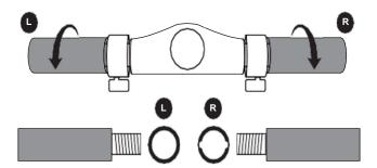
Please make sure to differentiate the left and handles carefully before installing the handles. Check the markings on the handles.
