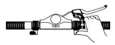
3. To stop riding You release the accelerator throttle and use the electrical brake to gradually decrease the speed and then step off the scooter one foot at a time. Please be cautious. Do not press the electrical button hard unless in emergency. Hard press of the electrical brake can cause abrupt stopping. Take time to familiarize yourself with the brake.
