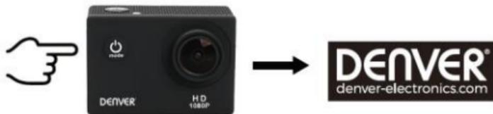
3.2 Power off: Press Power key for 3 seconds when the camera is in the idle state to turn it off.
