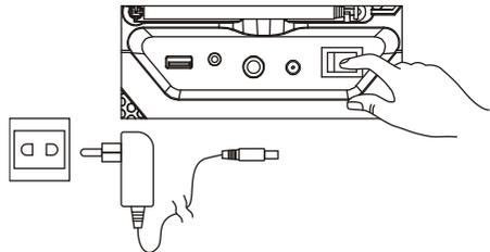
**It is recommended to charge the battery about 6 hours before you start using the unit for the first time.**
