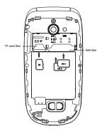
Inserting a memory card: in order to use camera and media player functions, a micro-SD memory card is required (not included in the package): the card must be placed into the rear of the phone to the left of the SIM slot. Insert the micro-SD card as shown, with the gold contacts facing downwards: open the metal shutter by pushing it towards "open" and lock it again after inserting the card by pushing it in the opposite direction ("close").
