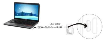
Connect the camera to the computer for charging, at this time, the charging indicator will be
